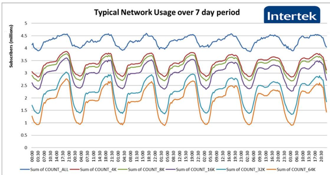
Figure 1. Network usage over a 7 day period, starting from midnight on a Monday, from the entire network infrastructure. The legend shows the specific thresholds mentioned above as 4kbps, 8kbps, 16kbps, etc. *Source: SEAD, 2014.*
